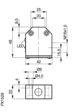
Inductive Sensors BES 516-346-H2-Y 22 x 42 x 48 normally-open Sn=5mm shielded
